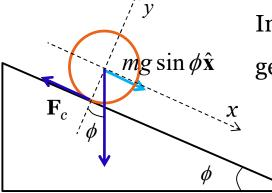
In this case, we need to go back to Newtonian mechanics to get the constraint force:
