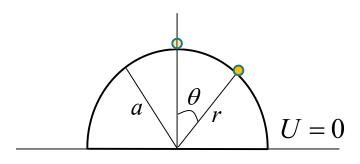
Problem: A point mass sits on top of a smooth fixed hemisphere with radius *a*. Find the force of constraint and the angle at which it flies off the sphere.
