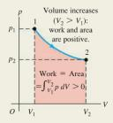
The first law of thermodynamics: The first law of thermodynamics states that when heat Q is added to a system while the system does work W, the internal energy U changes by an amount equal to Q - W. This law can also be expressed for an infinitesimal process. (See Examples 19.2, 19.3, and 19.5.)
