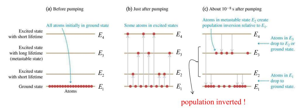
Over the next  $10^{-3}s$ , "enhanced" stimulated emission will then produce a coherent laser beam with frequency  $f = (E_3 - E_2)/h$ .
