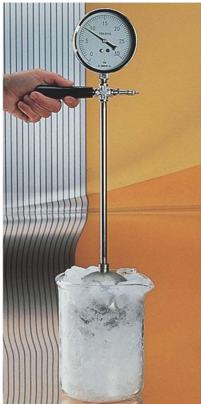
(a) A constant-volume gas thermometer
