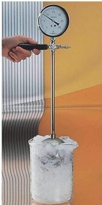
(a) A constant-volume gas thermometer
