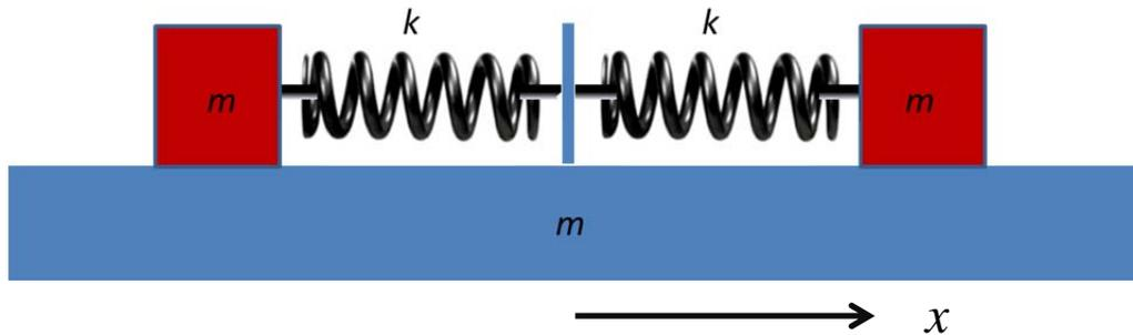
A platform of mass,  $m$ , is sitting on a frictionless surface and is free to move in the  $x$ -direction. Two identical blocks, also of mass,  $m$ , are connected to a thin massless post fixed to the platform by two identical massless springs of spring constant  $k$ . The blocks are free to move on the platform in the  $x$ -direction without friction.
