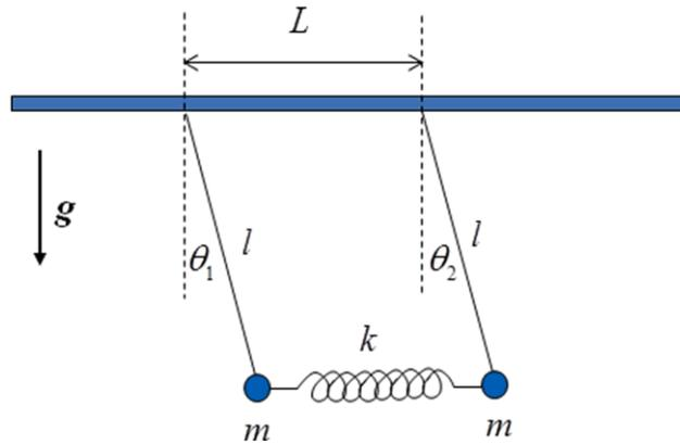
Two pendula with equal mass  $m$  and length  $l$  are connected by a spring with a spring constant  $k$ . The unstretched length of the spring is equal to the distance  $L$  between the support points of the two pendula. Considering small oscillations along the line between the two masses (consider only stretching of the spring horizontally and ignore the small vertical stretching), find the eigenfrequencies (resonant frequencies) and the normal modes for the system.
