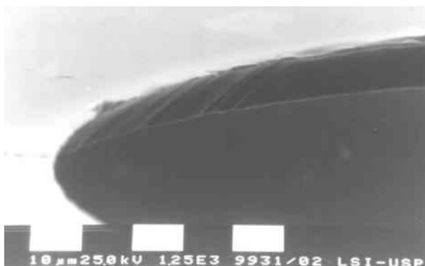
Fig. 1. A 450µm diameter circumference etched on a 13µm thick polyimide foil.
