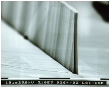
Fig. 1: SEM photograph of a monocrystalline 2 \mu\text{m} -wide vertical wall made on silicon.
