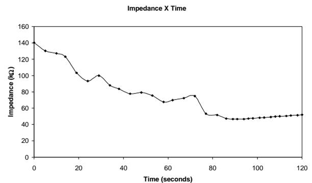
**Fig. 8: Microelectrode impedance variation as a function of time.**
