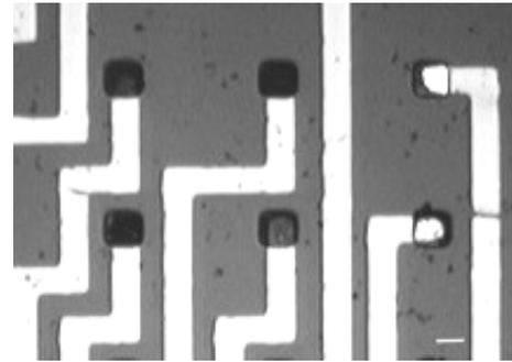
**Fig. 7: Visual evaluation of track and electrode state, passivation and platinization (image from the optical microscope).**
