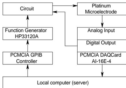
**Fig. 3: Setup block diagram.**
