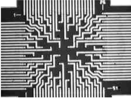
**Fig. 2: Display of the manufactured microelectrodes array central area (1mm<sup>2</sup> in the picture), with 120µm space between adjacent electrodes.**
