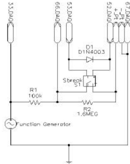
**Fig. 4: Circuit diagram for current limiting during platinization.**
