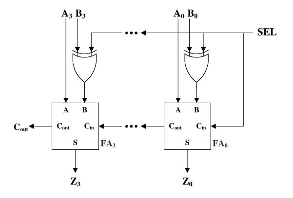
The circuit diagram above implements a 4-bit adder-subtractor:
